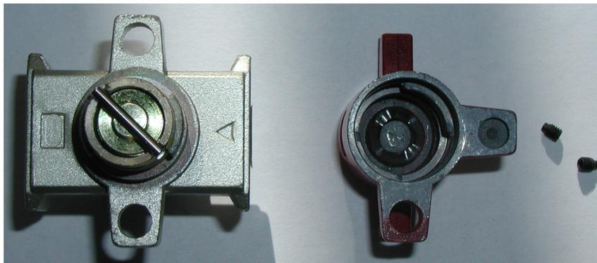
2. PUT CAP PIN ON TOP OF THE SPRING CAP AND ALIGN WITH THE SLOT OF THE VALVE BODY
